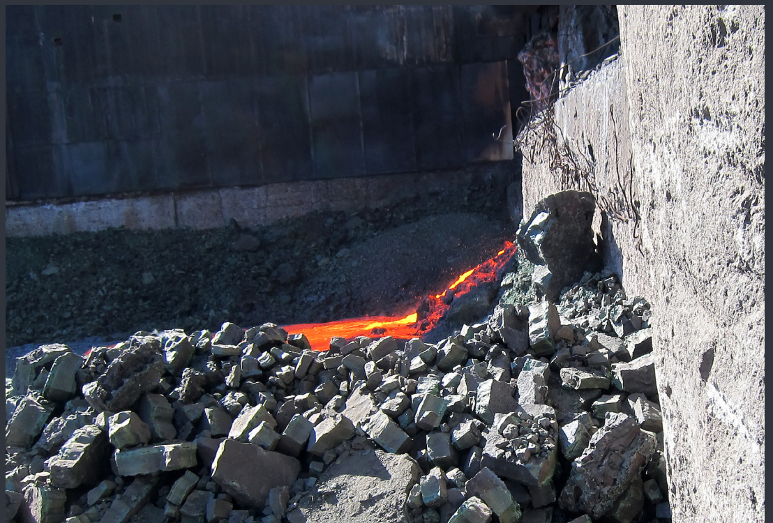
When water is used to cool hot slag, its temperature rises. The heated waste water is reused to flush out the filter.
